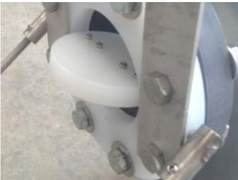
These float valves have a correct installation position and an incorrect position. If installed upside down- the operation will be reversed (the valve will close when the float position is down). If this is the case- remove and re-install the valve in proper position.
