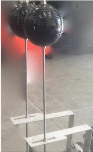
The Vertical Float valve is designed for water level control above the surge tank inlet flange and is traditionally used to modulate the flow of main drain water flow based on surge tank water level. Maximum operating range is 15”-58” above the valve would be standard, but this can be adjusted by sliding the floats down the rods to reduce this range if required.
