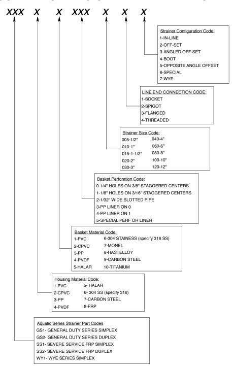
TO IDENTIFY YOUR PARTICULAR STRAINER, USE THE ABOVE KEY TO DETERMINE CORRECT STRAINER MODEL. STRAINER MODEL IS ALSO PROVIDED ON THE EQUIPMENT IDENTIFICATION TAG AFFIXED TO THE STRAINER HOUSING.
