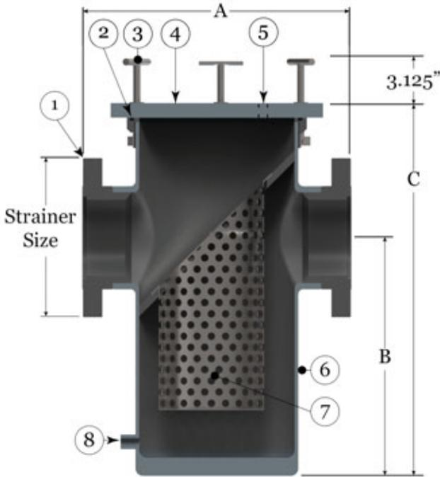
The Fluidtrol GX Series is a non-metallic housing inline basket strainer engineered for general water through moderately corrosive industrial water systems.
