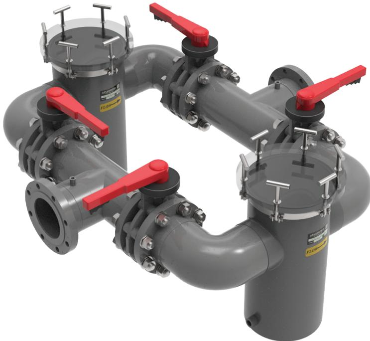
Duplex strainers are a good choice for critical systems for which flow interruption is prohibited. A properly designed composite duplex strainer assembly will allow full flow through one strainer, while the other is isolated and in standby with a clean basket in place. Monitoring the pressure drop via optional pressure taps on inlet/outlet manifold allows for easy identification of when basket becomes fouled and changeover is required.
