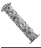
The standard basket will be the same material as the plastic liner with 1/4 perforations. Select your basket by first determing the opening size. Next determine the material most suitable for your fluid. SS316 has the best availability. AL6XN is great for salt water. Hastelloy C276 and Monel are sutiable for many fluids and a good option when mesh liners are required. PVC fairs well upto 140 deg F, PP and CPVC 180 deg F, and PVDF 250 deg F.
